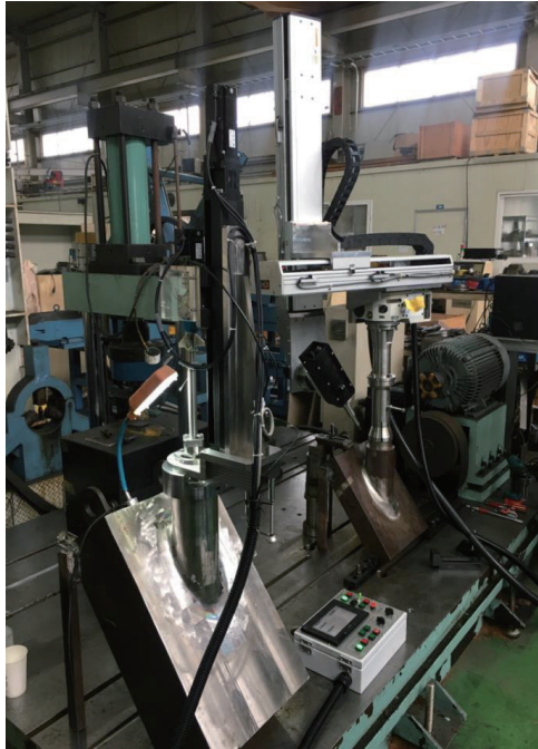
Figure 8. UNSM equipment on CRDM nozzle mockup.
