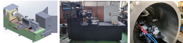
Fig. 5. UNSM device and UNSM unit for Main Steam nozzle
